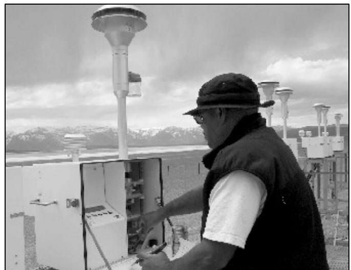
Technicians collect dust samples weekly from remote, solar-powered equipment. The data are critical to understanding air quality trends.
