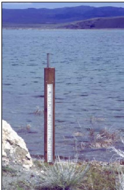
May 1998, the newly installed lake level gauge—in anticipation of the lake's rise. Lake level: 6383'
