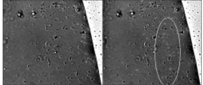
*This image shows a before (left), where all of the magnetic bacteria are collected at the edge of a drop (the dark area). On the right is the same drop, a few seconds after reversing the field direction. There is a wave of magnetic bacteria swimming away from the drop that are highlighted by the white circle.*
