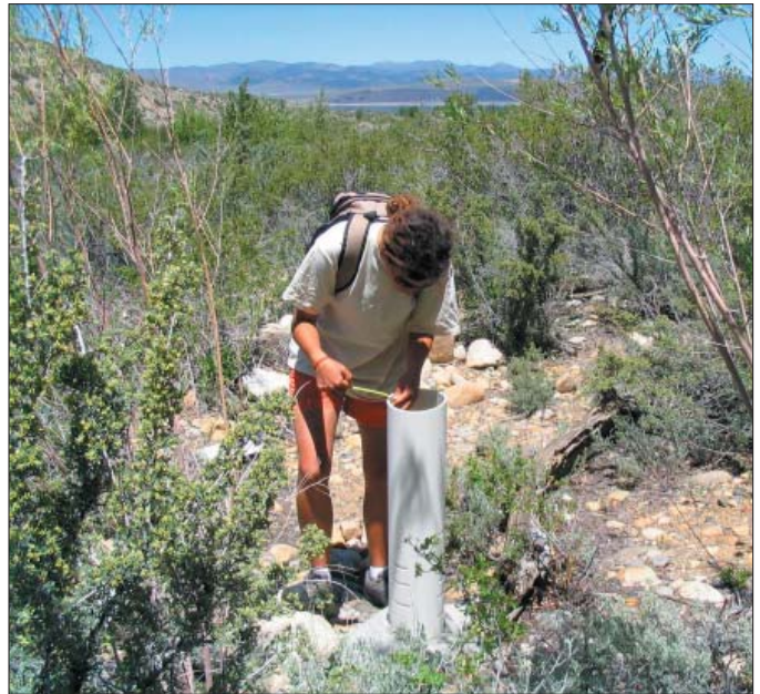
Committee staff record piezometer readings, measuring groundwater levels at key points around the Basin.
