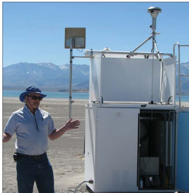
Specialized air quality monitoring stations are necessary at Mono Lake to measure the frequency and severity of dust violations.
