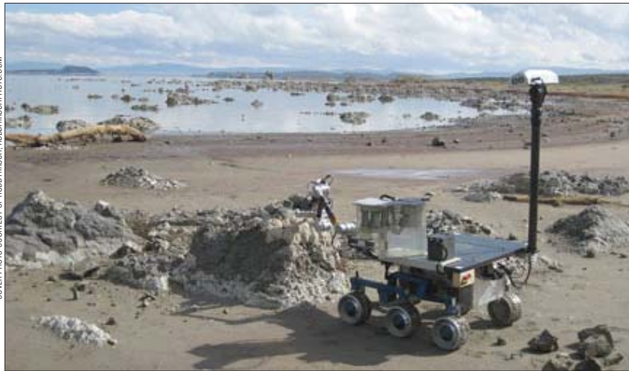
In October the Jet Propulsion Laboratory and NASA brought a prototype Mars rover to Mono Lake to field test its rock-sampling procedures and equipment.
