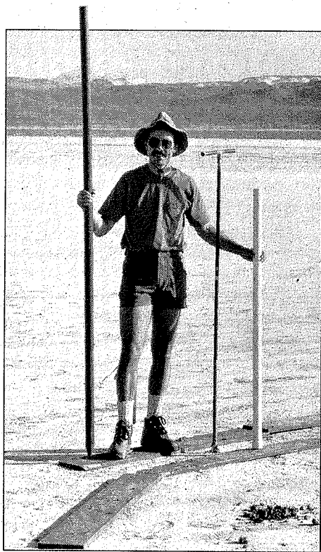
A piezometer is a piece of tubing open at some depth to allow ground water in from the surrounding soil. Using an auger, David Rogers is installing several at Ten Mile Road in the project to track seasonal and spatial variations in groundwater levels and quality at Mono Lake.
