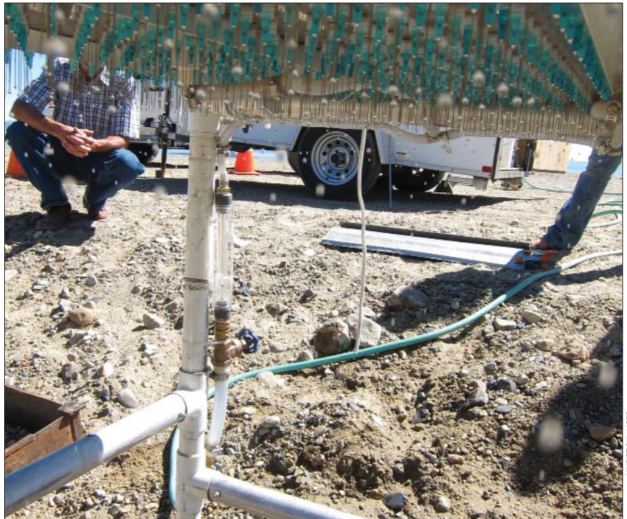
This rainfall simulator was used to test runoff quantity and quality from vegetation test plots as part of the revegetation project at the Lee Vining Airport.
