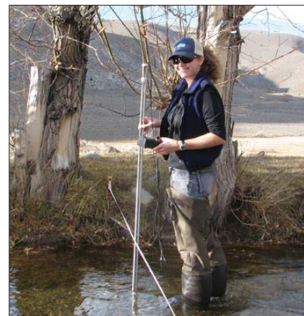
Project Specialist Emma Oschrein measures flow in the Lundy hydropower plant tailrace.
