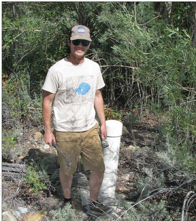
Mono Lake Intern Matt Rice measures groundwater levels adjacent to Mono Lake's tributary streams using piezometers (the white pipe pictured above).
