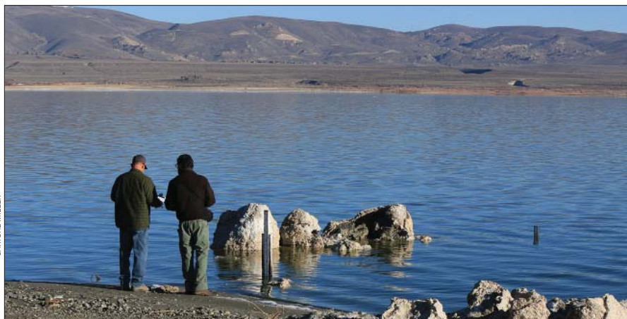
DWP and Mono Lake Committee staff read the lake level gauge together every April 1. The lake level is one, but not the only, component used to determine DWP's allowable water exports for the year.
