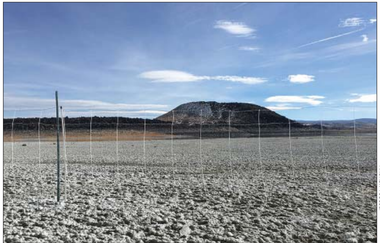
In December, the Committee and partners put up a test fence on the landbridge and determined that the mesh netting stands up well to the elements.
