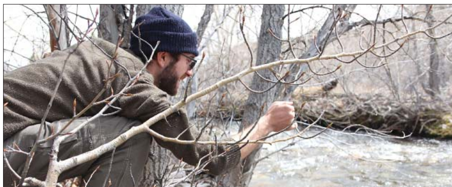
Robbie places a temperature recorder into Lee Vining Creek that will collect data all summer.
