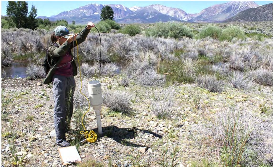
Caroline measures groundwater in a piezometer on Rush Creek as part of stream restoration monitoring.
