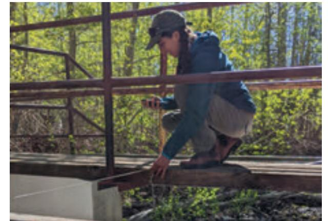
Zoe measures and records Mill Creek streamflow as part of north basin restoration monitoring.
