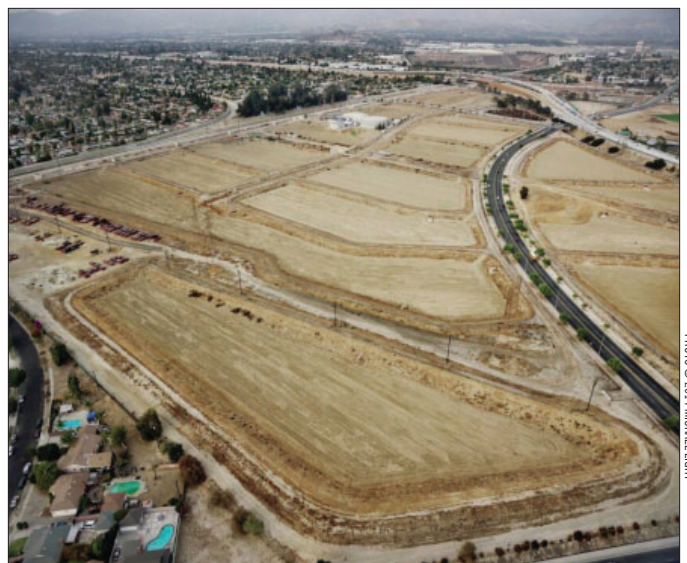
DWP’s Tujunga Spreading Grounds, which capture stormwater and recharge the San Fernando groundwater basin with 16,000 acre-feet of water annually, is great example of increased local water capture.
