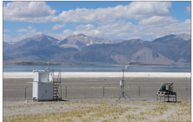
New DWP air quality monitoring equipment (center, right) next to Great Basin's long-established, better-quality equipment (left).
