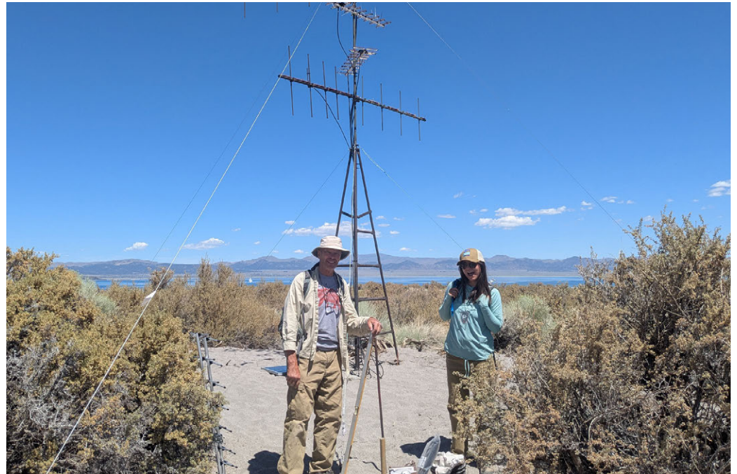
The Committee installed three Motus towers around Mono Lake this year. Part of a global network, the technology helps scientists understand the migration routes of tagged animals like Wilson's Phalaropes.
